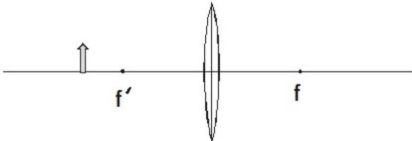
9. A double convex thin lens has a focal length of 50.0 cm. A 2.70 cm tall object is placed 18.0 cm from the lens, find (a) the image distance, (b) the magnification, (c) the image height.
